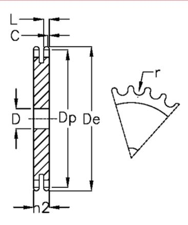
C = 2 D = 30 De = 700.6 Dp = 691.36 For chain size =  $3/4 \times 7/16$ For chain type = 12 B-2 h2 = 30.3 L = 10.8 Number of teeth = 114r = 12.07
